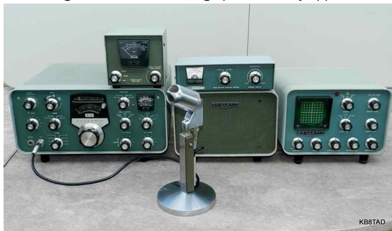
Heathkit SB-101 Station – everything (except the microphone) was assembled from a kit, but Heathkit stopped offering kits in 1992.
