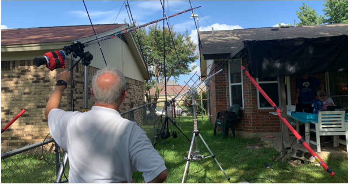
N5HYP pushing his antenna stack manually while Guy, K5GBD watches his antenna rig track the same satellite.
