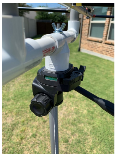
Close-up view of antenna/tripod mount. Note tripod level indicator
