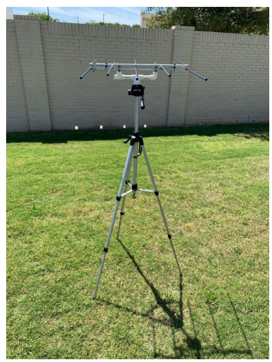
Completed Tripod with Elk 2m/44L5 Antenna, horizontal polarization
