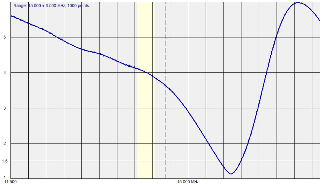
Figure 5 Graph of my badly mis-adjusted 20 Meter antenna elements as drawn on PC software
