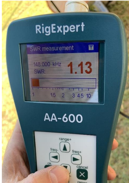
Figure 4 Real time SWR reading at 148.000 MHz
